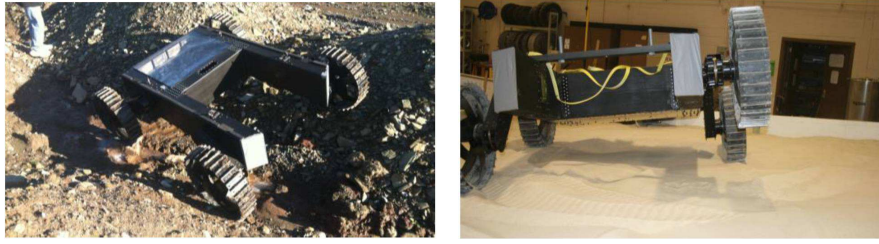
Fig. 6 Field tests (left) led to the discovery and study of suspension lift-off (right).
