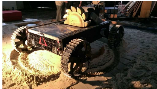
Fig. 5 Polaris excavator featuring continuous bucket-wheel excavation and high payload ratio.
