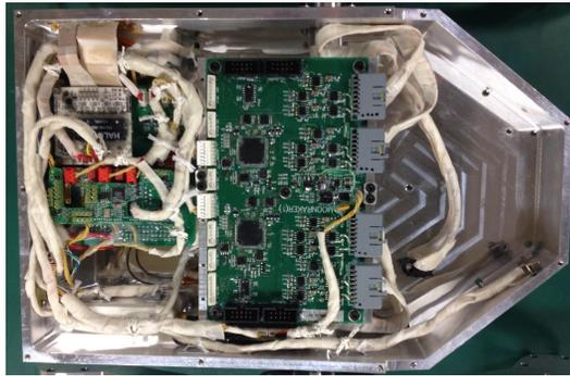
**Fig. 9** Moonraker's internal components, with complex wiring harness.
