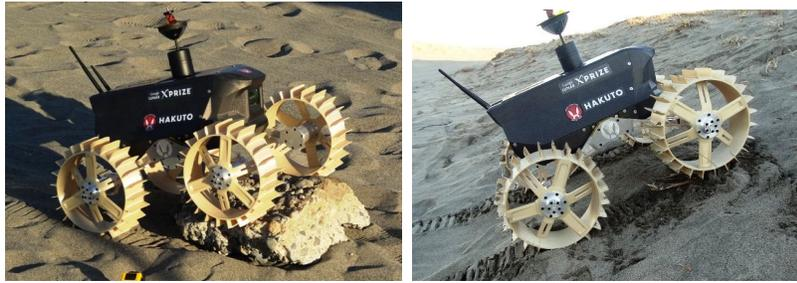
(a) overcoming a 15 cm high rock obstacle during field testing (b) climbing an approximately 30° slope on soft soil
