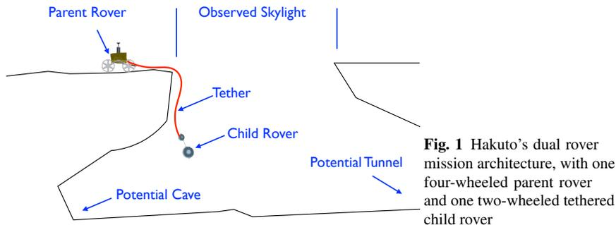
**Fig. 1** Hakuto’s dual rover mission architecture, with one four-wheeled parent rover and one two-wheeled tethered child rover
