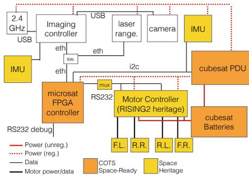
**Fig. 4** Moonraker Architecture for Phase Four of Development
