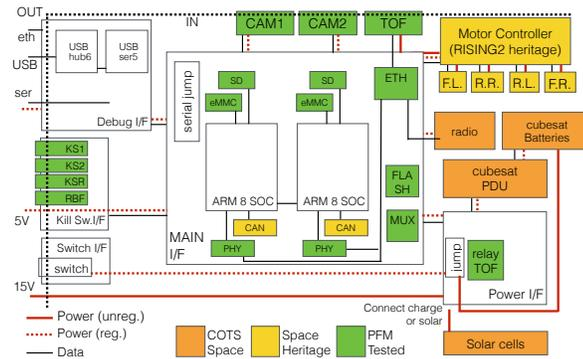
**Fig. 10** Moonraker Flight Model architecture
