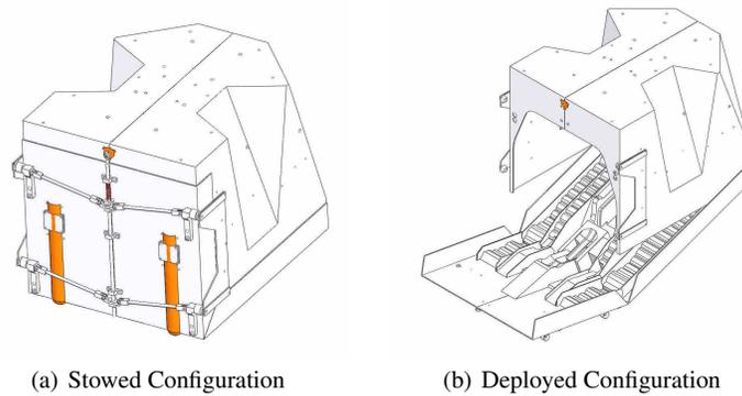
**Fig. 5** View of the interface box. Moonraker and Tetris are nested inside when stowed. When deployed, the door forms a ramp for the rovers to drive down
